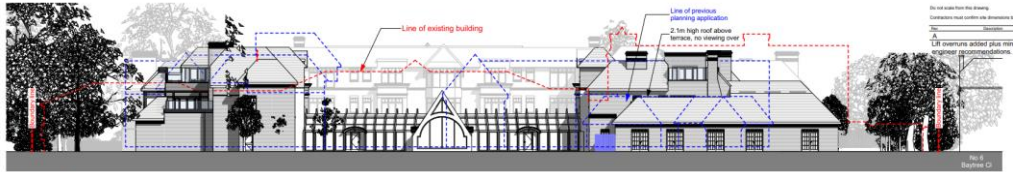
Fig 7. Proposed rear elevation facing High Grove (red line indicates existing building. Blue line indicates previous dismissed scheme).
