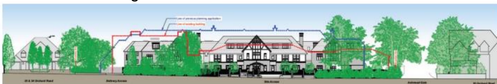
Fig 3. Proposed front elevation (Red line indicates existing. Blue line indicates previous dismissed scheme)
